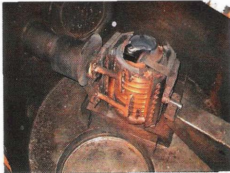
Fig. 2. Induction furnace in vacuum chamber
