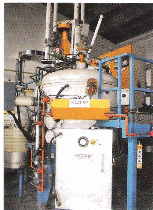
Fig. 1. Vacuum casting furnace
